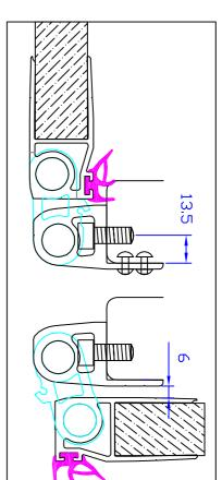
should be placed above and below each hinge using Section showing hinge arrangement in closed and 270° open positions. Fix hinge support profile to pillar using 2 alternating rows of rivets at 250mm centres along the two drilling lines. Additionally for heavier duty applications, M8 caphead bolts the holes provided.
