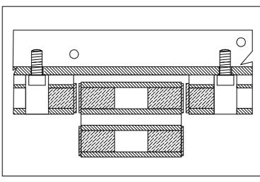
hinge rod in support profile using pins provided. Ensure pin held securely both ends and seal/fill pin holes with sealant. open 90° NB shorter open 90° NB shorter plastic bush in support profile. Drill and pin (min. x2) to secure 12mm Side view section hinge support, hinge blade 6.5
