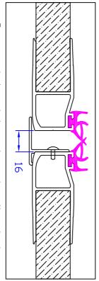
Ensure central gap between doors at meeting edge is correctly and consistently set.
